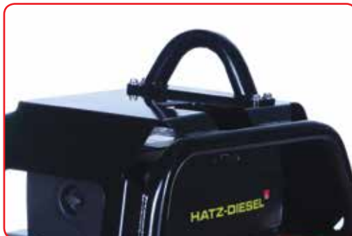
Central Lifting Hook for Easy Transportation
