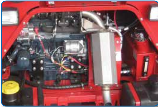
High Horse-Power KUBOTA® V1505-T for Maximum Power and Performance: : A Naturally-Aspirated Engine Complying to EPA Tier 4, EU Stage III-A Emission Regulations 3-Cylinder Liquid-Cooled Diesel Engine, JAPAN
