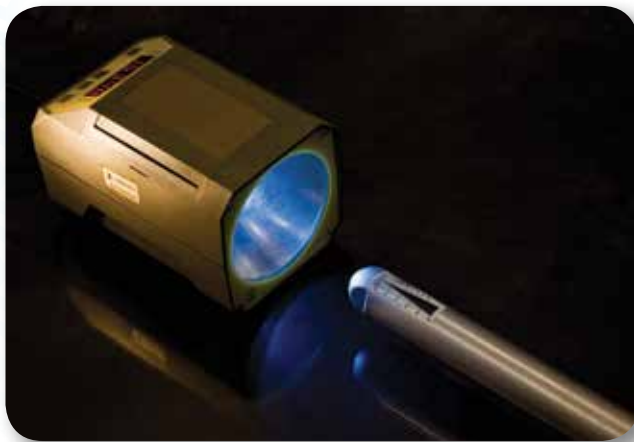
Stroboscope is used to Measure the Vibration Frequency and the Rotational Speed of the Vibrator Head
