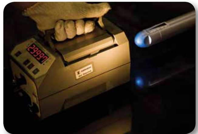
Stroboscope is used to Measure the Vibration Frequency and the Rotational Speed of the Vibrator Head
